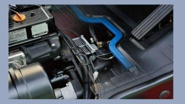
1. In addition to rubber damper between overhead and frames, compound engine damper and full floating power train achieve flexible connection between frames and driving system, as a result, traveling vibrations and vibrations from the driving system are significantly reduced.
