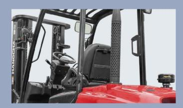
**4.** The new design mast provides broad forward visibility due to the longer distance between inside mast.
